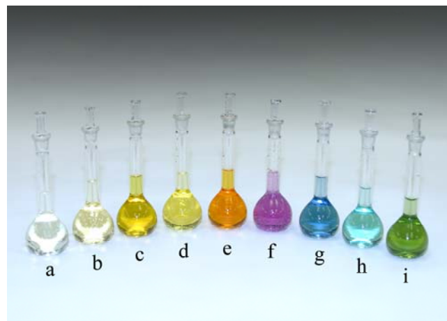
Figure 2. Photograph of solutions produced in the current experiment. Solutions are ordered according to the ligand spectrochemical series: (a) \text{CN}^- , (b) \text{NO}_2^- , (c) phen, (d) en, (e) \text{NH}_3 , (f) gly, (g) \text{H}_2\text{O} , (h) \text{ox}^{2-} , (i) \text{CO}_3^{2-} .
