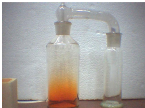
Figure 1. Diffusion of bromine in air, the equipment used, and the beginning of the experiment.
