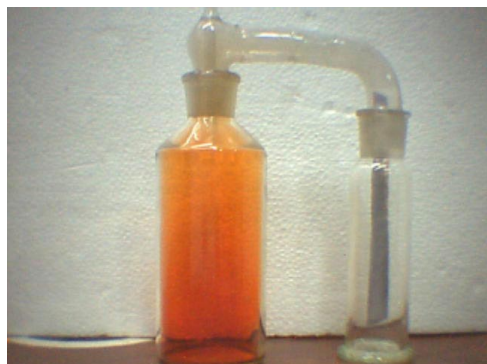
Figure 2. The diffusion of bromine progresses; the paper soaked with a solution of KI and starch turns blue.
