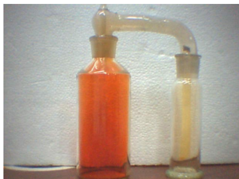
Figure 3. Diffusion of bromine; with excess bromine, the paper is discolored.
